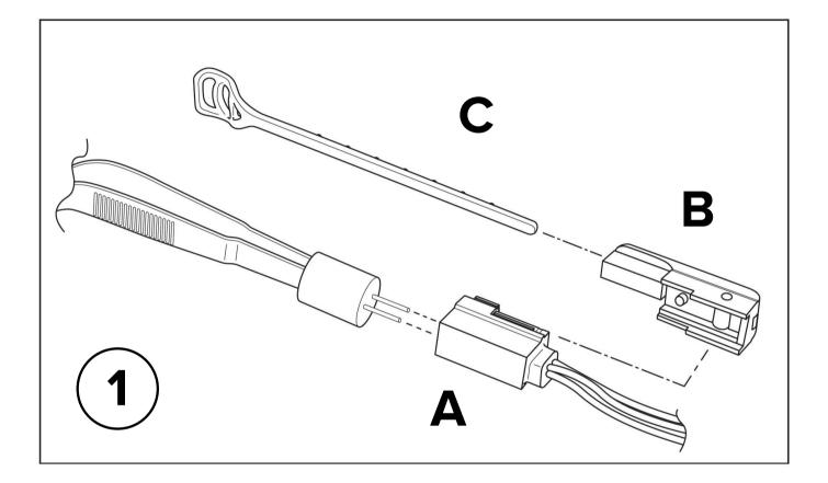
Drawing 1: The forceps are connected to the inserted into forceps plug (A) end of the BiPAD cord.
