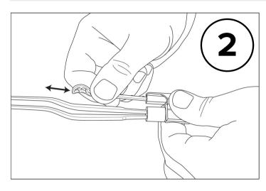
Drawings 2 & 3 show that the external arm ( labeled (C) in drawing 1 above ) can be shortened or lengthened by sliding in and out.
